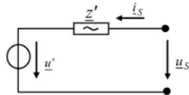
Figure 2 Quasi-stationary equivalent circuit of the DFIM.
