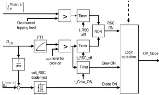
Fig. 6. Switching logic between different operating modes.
