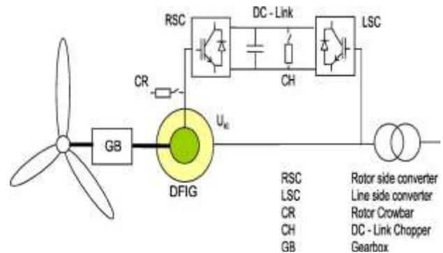
**Figure 1 Structure of the DFIG-based wind turbine system.**
